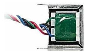
These transformers are great for allowing crystal radios to use low-impedance headphones. They are also perfect for the laser communicator project, and the AM transmitter project. They convert 8-ohm impedance to 1,000 ohms. The 1,000 ohm side is center tapped.
