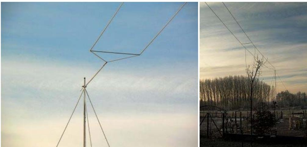
Electrically the Marconi antenna is nothing more than a vertical antenna with a tip that splits and goes horizontally, making a hat. This configuration gives great performance on low frequencies, and for this reason it is also widely used by the military to transmit signals in the VLF band.
