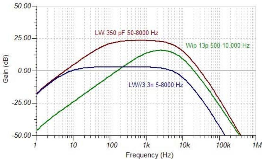
The graph, which is purely indicative shows varied frequency responses. Represented here are the curves of gain between the voltage detected by the antenna and the output voltage to the LINE output jack of the receiver with three different antennas:
