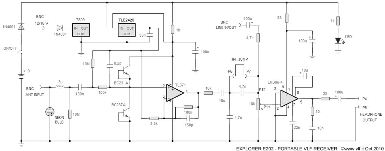
The second stage consists of a low impedance amplifier (LM386-4) to drive a headset which is perfect for "live" field listening. The jump HPF short-circuits a capacitor that acts as a high-pass filter. Removing the jumper between pins 6 and 7 activates a high-pass filter that attenuates low frequencies such as 50 Hz by about 30 dB. You can build it as a jumper on the board or as an external switch on the receiver box.
