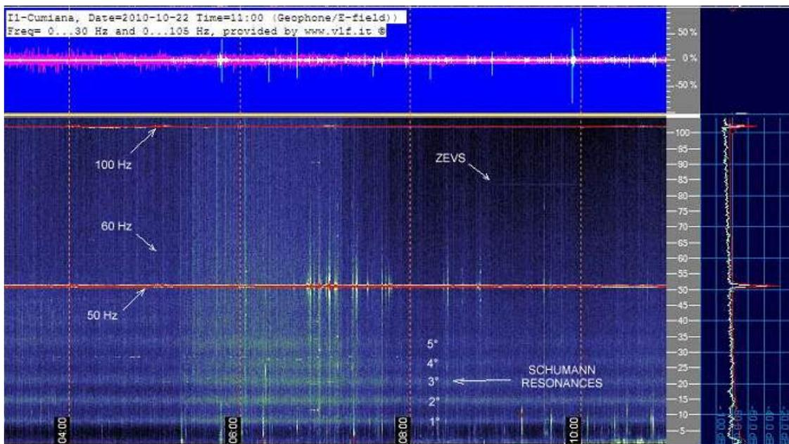
In the spectrogram above, developed with SpectrumLab and obtained on a received signal with a Marconi wire antenna, are visible: the Schumann resonances, a 82 Hz Zevs signal from a Russian submarine broadcast network, 50 Hz network, the first harmonic at 100 Hz and the weak 60 Hz signal of American power grid.
