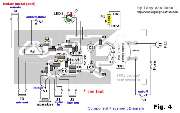
Components not shown on the printed circuit board are mounted on the front and rear panel of the enclosure.
