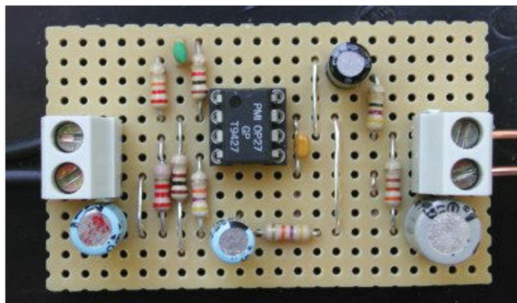
Figure 3. The amplifier circuit
