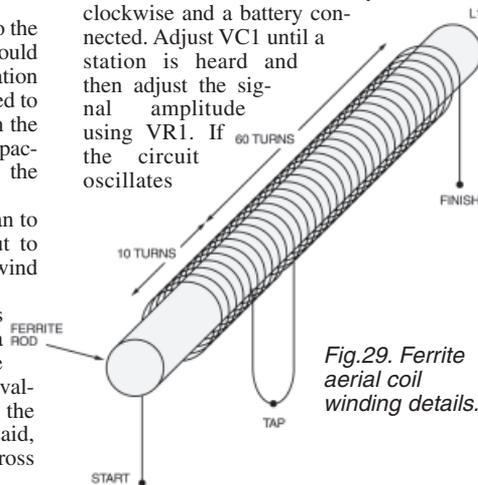
Fig.29. Ferrite aerial coil winding details.
