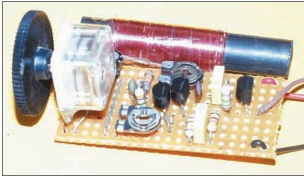
Completed radio showing the ferrite rod aerial.
