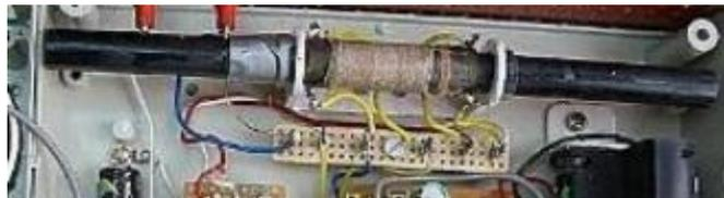
But as the ferrite rod antenna was placed near the rear panel, we have changed this one for a plastic sheet that does not shadow the electromagnetic waves.
