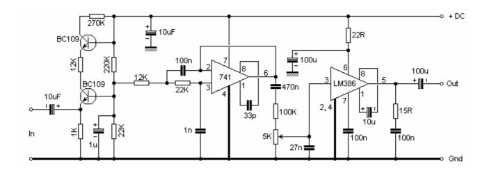
Audio taken from your receiver is fed to the pre-amp which consists of the two BC109 transistors and then passed to the 741 op-amp. This is configured as a Butterworth filter centered around 500Hz.
