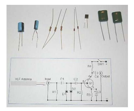
You can place a capacitor across R1 for a wide-band general tuned circuit. You can remove R1 for a sharply tuned circuit.
