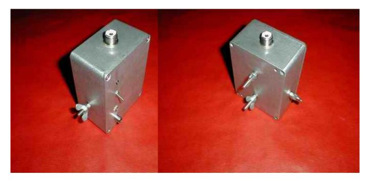
The two screw's at the back is for mounting a aluminium tube to set into the ground and the screw at the left side are for ground cable if used, antenna are a one/two meter 8 mm aluminium tube. mounted in a PL 259 male connector with some 10 mm air hose as isolator and some crimp flex to complete the finish, I have made two antennas the first at one meter and the other at two meter to use at more silent areas.
