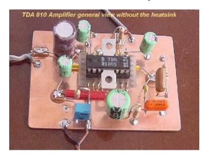
...built around the TBA 810 Integrated Circuit
