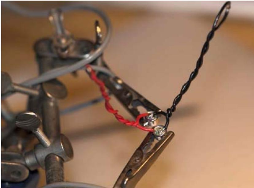
wiring of two capsules together in parallel
