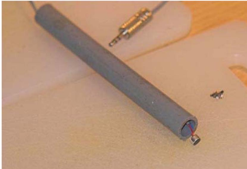
The capsule fitted to the wire is now threaded through the tube,
