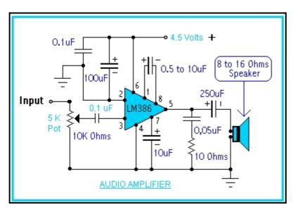
This receiver can be operated directly with a high impedance earphone, a crystal or ceramic earphone...but adding to its output an audio amplifier makes the set a complete radio receiver able to drive any 8 ohms 0.2 watts speaker.
