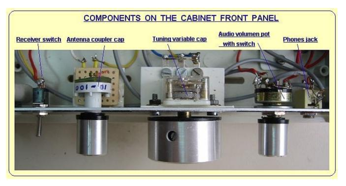
We have situated the external antenna variable capacitor at the left of the front panel; just near the receiver switch. At the right is the volume audio control potentiometer, near a jack for the phones, and in the center is the tuning variable capacitor. At the rear panel of the cabinet are two jacks, one for the exterior antenna and other for ground. Having the main knobs and switches in the front panel is quite easy and a pleasure to command the receiver.
