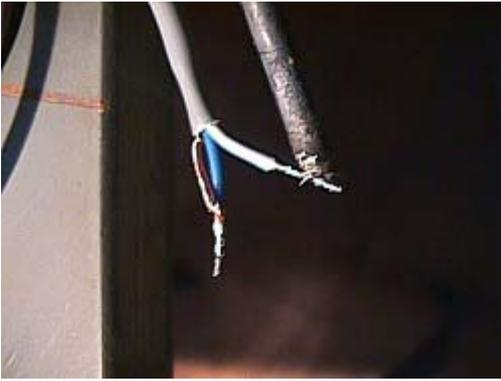
Twist one of the wires together with the ground wire, and tin the ends of the wire with solder. Do this on one end only. On the other end of the cable, cut off the ground wire so that only the two insulated wires are exposed.
