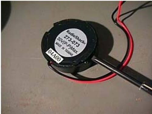
Use a thin edge (screw driver, xacto blade etc.) to gently pry the back plate off of the packaging. Careful not to bend the visible brass PZT disc
