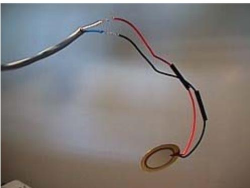
Tin both wires on the other end of the cable. Put two short pieces of heat-shrink tubing on the PZT leads. Solder wires together. I prefer to do this by lining up two tinned leads side by side. Some people prefer to twist the wires together before tinning and soldering.
