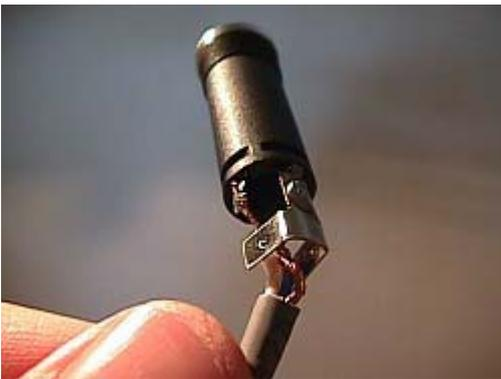
Unscrew the housing from a 1/4" jack. Solder the ground wire to the large contact, and the 'signal' wire (white) to the contact point (see below). Careful not to melt the cheapo connector. Also, be careful to make sure your solder wycks on the surface of the contacts, meaning that you have a good solder joint.
